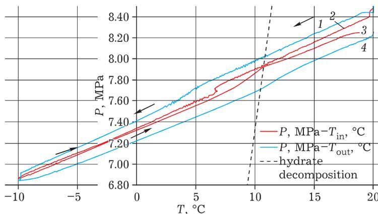
Fig. 3. Course of a typical experiment: 1 and 4 – pressure in the autoclave collated with the temperature of the heat-carrier; 2 and 3 – the same in the centre of the autoclave; curves 1 and 2 describe the stage of lowering the temperature and formation of gas hydrates; curves 3 and 4 – increase accompanied by their decomposition.
