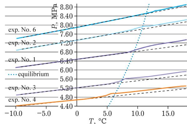
Fig. 4. Decomposition of methane hydrate. Curves of pressure change compared with the temperature inside the autoclave for the stages of increasing the temperature in exp. Nos. 6, 2, 1, 3 and 4, respectively (see Table 2). The equilibrium curve of methane hydrate is also shown.
