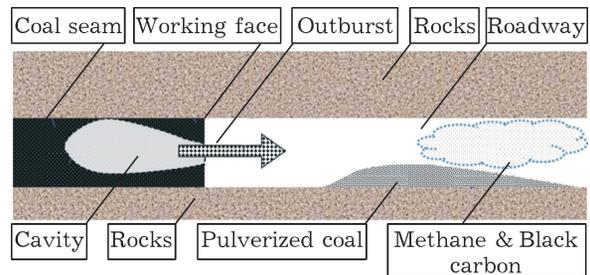
Fig. 1. Sudden outburst of coal and gas in a coal mine.
