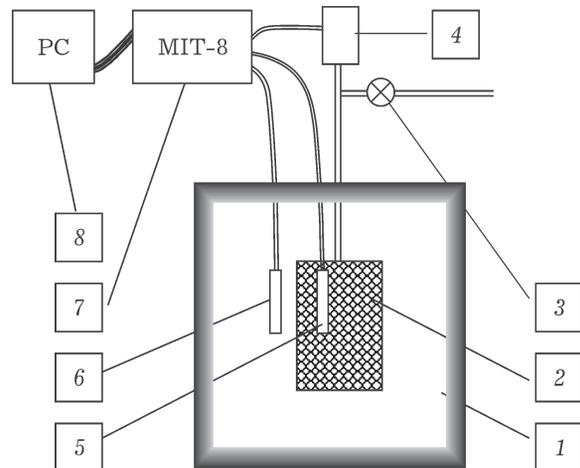
Fig. 2. Scheme of experimental setup: 1 – thermostat; 2 – autoclave with coal and gas; 3 – gas valve; 4 – pressure transducer; 5, 6 – temperature transducers installed inside and outside the autoclave; 7 – multi-channel measure MIT-8; 8 – PC (personal computer).
