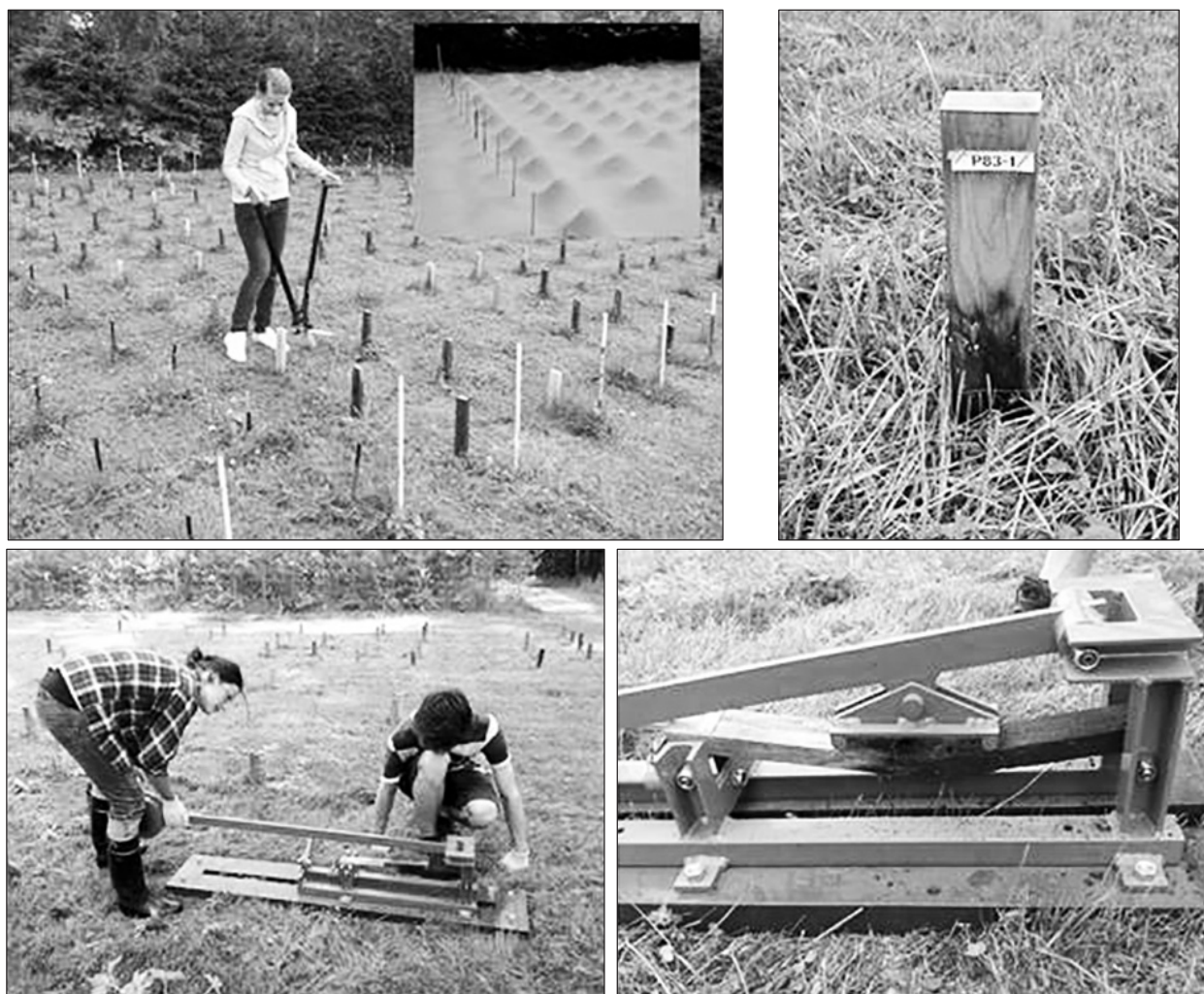
Fig. 3. Overall view of EN 252 decay field test at Punkaharju in summer and winter time, grass maintenance, Scots pine stake in close view and strength measuring with a bending apparatus.
